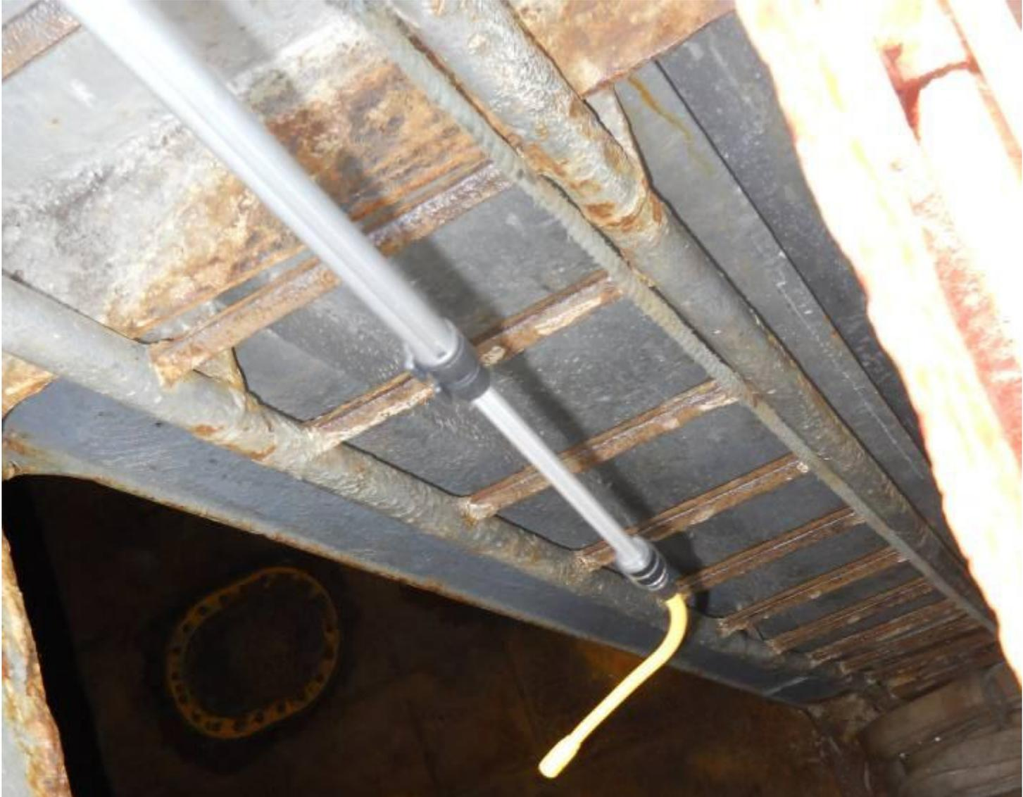
It is necessary to obtain a reading for the level of ultrasound reaching the underside of the cargo hatches.
